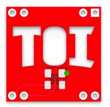
**WARNING**: Component labels on this badge are a little confusing, THE LED is on the TOP, the RESISTOR is on the BOTTOM. Don't mess it up!
